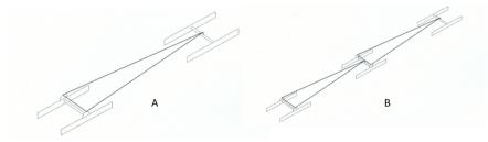
When using MJT CCUs on a conventional coach (A), stabilisation of the body is achieved by the etched semi-circular 'triangulation tabs' on one of the bogies. The other bogie is free to pivot in any direction. With an articulated set (B) this principle must be replicated throughout all the vehicles. The articulated bogie must act as the 'free' bogie for one vehicle and the stabilising bogie for the next.
